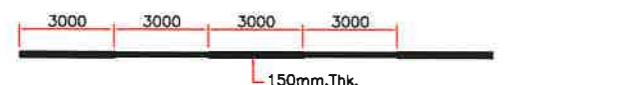
LANE MARKING FOR 2-LANE ROAD ON CURVES AND APPROACHES TO INTERSECTION IN URBAN AREA (RM-05B)
